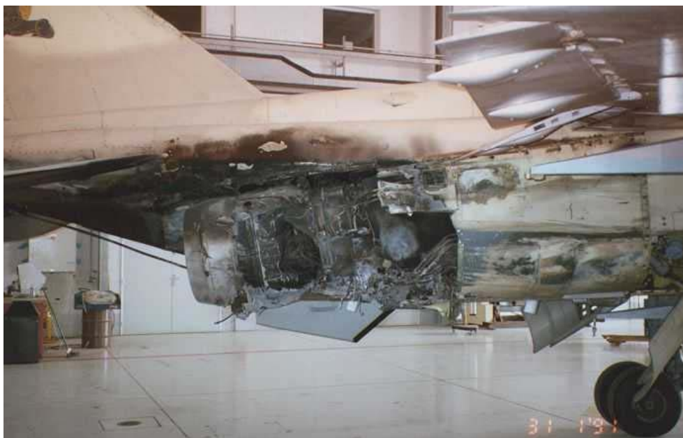
Figure 2: Damage inflicted on a Jaguar Aircraft during the Gulf War by a small SAM (MANPAD). Typical missiles of this type have warheads of less than 1kg and an “all burnt” mass of less than 10kg. Photograph courtesy of RAF ABDR Flight, St Athan.
