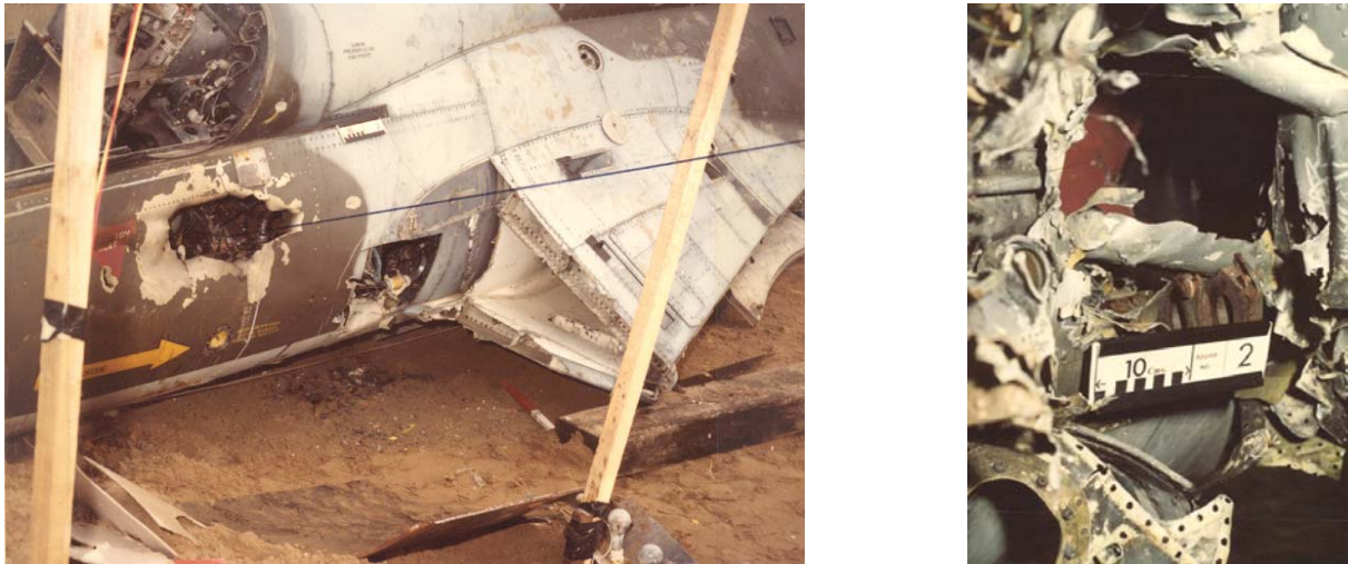
Figure 4: Direct Hit Damage to Aircraft Fuselage. This level of damage was assessed as causing a permanent loss of flight capability within 5 minutes (UK F 5MIN kill category).
