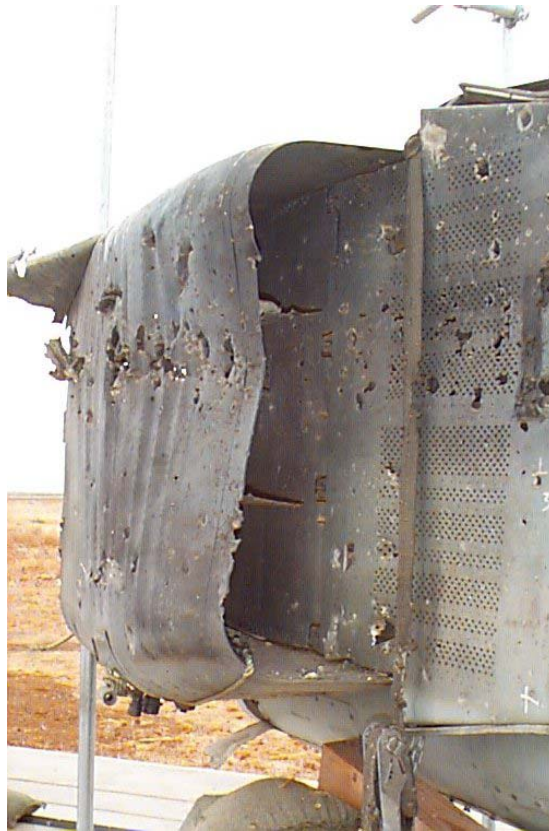
Figure 1: Typical Close Burst Damage to a Mig 23 Aircraft. The fragment swathe struck the intake first, weakening the structure, which was then distorted by the blast loading. The photograph was taken during a joint Dstl/DSTO trial conducted at the Port Wakefield test range in South Australia.
