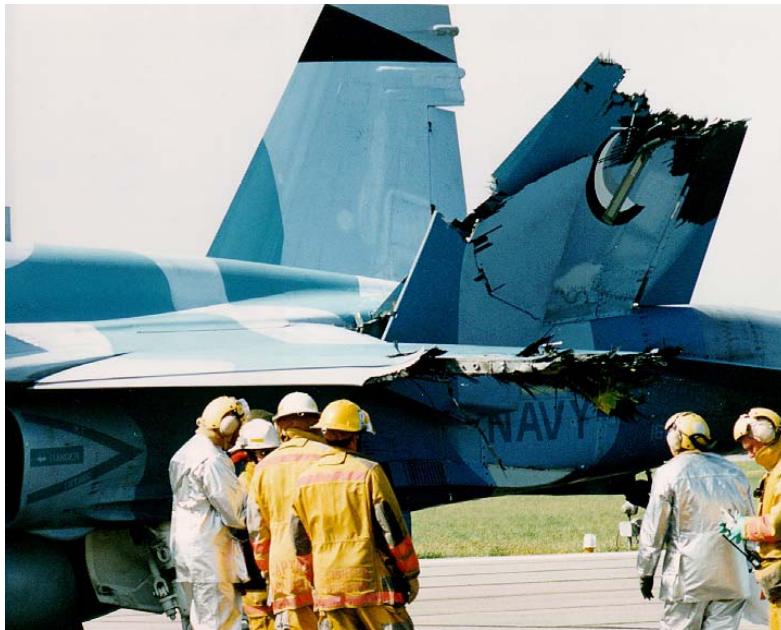
Figure 3: “Survivable” Damage as a result of a Mid Air Collision. Approximately 50% of the port wing has been removed along with a large section of the port tail fin. The fin has also suffered severe damage to its primary structure.
